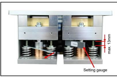
If an adjustment is needed turn the M6 nuts using the spanner provided. Adjust all springs on both sides equally. Moving the spanner to the left raises the units.
