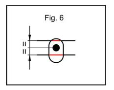
Figure 6 shows the optimum adjustment where the pin is situated **midway** between the two lines.
