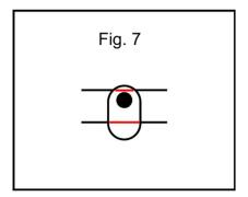
When the pin is just tangential to the lines as shown in figures 7 and 8 the system is still floating but with only 0.5mm free movement, downwards or upwards respectively.
